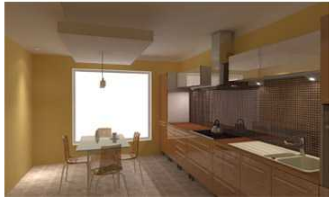
After the adaptive mesh division – artificial shadows between the walls and the ceiling are gone
